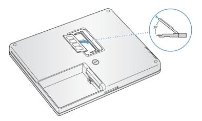
6 Press down on the memory card to lock it in place. If the memory card does not latch, do not force the card down. Try reinserting the card to make sure it is fully seated.
