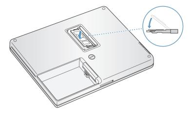
7 Replace the memory slot door and screw it into place.
