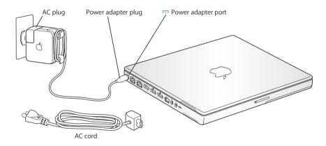
To extend the reach of your power adapter, you can attach the AC cord if desired. See "Using Your Power Adapter" on page 23.
