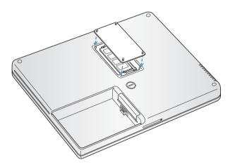
*Note:* To avoid damage, be careful not to overtighten the screws.
