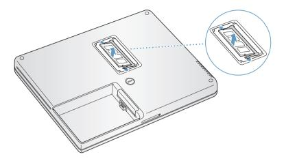
5 Insert the new memory card into the slot at a 30-degree angle. Push the card to seat it fully into the slot.
