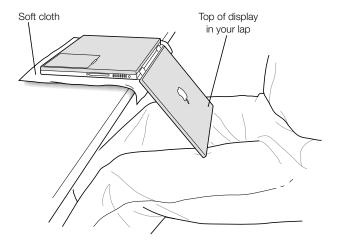
**Important** Do not open the display further than the angle shown above.
