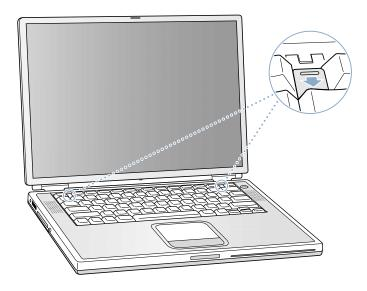
Lift the top portion of the PowerBook keyboard up slightly near the top row of keys and pull it back far enough to displace the small tabs that hold the bottom of the keyboard in place.
