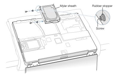
4 Insert the right side of the drive first, then insert the left side of the drive. Use the holes in the drive carrier to line up the drive with the bracket.
