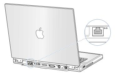
Connecting to a network gives you access to other computers. You may be able to store and retrieve information, use network printers, modems, and electronic mail, or connect to the Internet. You can also use Ethernet to share files between two computers or set up a small network. The Ethernet port on your PowerBook auto-detects other Ethernet devices. You don't need an Ethernet crossover cable when connecting to other Ethernet devices.
