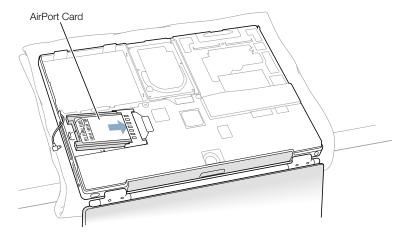
5 Connect the AirPort Card to the end of the antenna cable.
