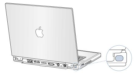
You can use infrared to share files with another IrDA-equipped computer, communicate with other infrared devices such as handheld organizers, connect to an infrared network, and even print on an infrared printer. Sharing files using infrared is the same as sharing files using Ethernet, except that AppleTalk and TCP/IP are set to Infrared instead of Ethernet. File sharing and IrDA printing are not supported in Mac OS X.
