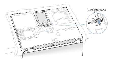
7 Attach the bottom case to the computer and replace the eight screws in the order shown in the illustration below.
