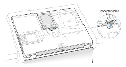
10 With a Torx T-8 screwdriver, remove the two screws that secure the hard disk carrier to the mounting bracket and then gently remove the hard disk.
