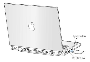
**Important** The Apple AirPort Card is installed in a slot inside your computer. It does not go in the PC Card slot the way many third-party wireless cards do. The AirPort Card will not work if it is installed in the PC Card slot and will cause your computer to function improperly.
