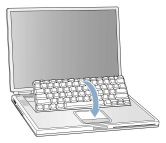
6 Flip the keyboard over and lay it on the palm rests and trackpad.
