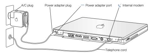
2 Plug the power adapter plug into the power adapter port (marked with the icon ---) on the back of the computer.
