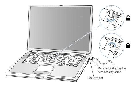
The keyboard locking mechanism is in the small plastic tab to the left of the Num Lock key, which also contains the Num Lock indicator light. Your PowerBook comes with the keyboard unlocked.
