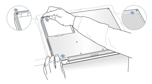
**7** Pivot the bottom case up as shown in the illustration below.
