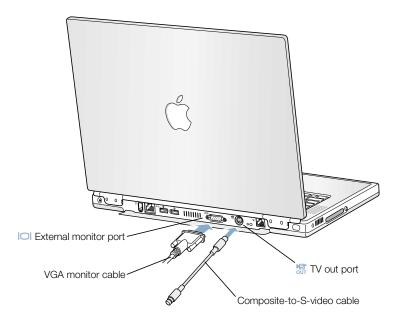
When an external monitor or television is connected, you can either have the same image appear on both the internal display and the external monitor (known as *video mirroring*) or use the external monitor to extend the size of the Mac OS desktop (known as *extended desktop mode*).
