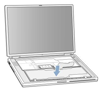
7 Touch a metal surface inside the computer to discharge any static electricity.
