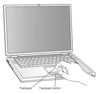
The trackpad is sensitive to how quickly you move your finger. To move the pointer a short distance across the screen, move your finger slowly across the trackpad. The faster you move your finger, the farther the pointer moves on the screen.
