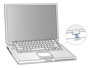
Pull down on the keyboard release tabs (located to the left of the F1 and F9 keys) and then press down on the top portion of the keyboard.
