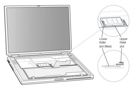
9 Hold the RAM expansion card at a 30-degree angle. Line up the notch in the card with the small tab in the RAM expansion slot. Then push the RAM expansion card into the expansion slot.
