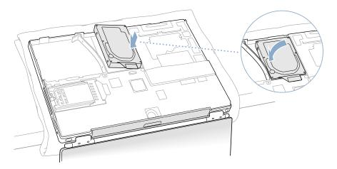
5 Lift the mounting bracket over the battery bay tab and lower it to its original position. Replace the screw in the top of the mounting bracket, being careful not to overtighten it.
