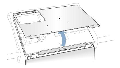
**Important** Do not twist the case from side to side. Slide the bottom case forward completely before lifting it up. If you feel any resistance when lifting the bottom case, double-check to make sure the bottom case is slid all the way forward and releases from the optical drive slot.
