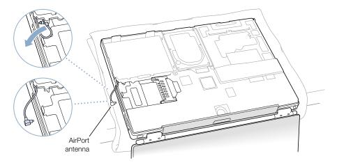
4 Position the AirPort Card with the AirPort ID numbers and bar code visible and slide the card into the connector.
