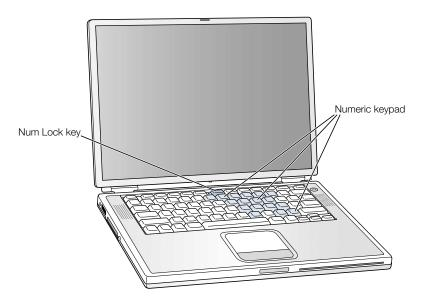
To use the numeric keypad, press the Num Lock key on the keyboard. The light next to the Num Lock key turns on, indicating that the keypad is active. When you're finished, press the Num Lock key again to turn it off.
