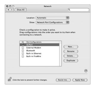
Next, follow the instructions to configure your network either manually or using DHCP, as instructed by your ISP or network administrator. If you're setting up your network yourself, it may be easier to configure the network using DHCP, because the server assigns IP addresses automatically.
