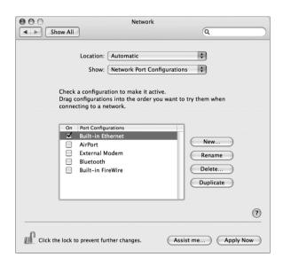
5 Drag Built-in Ethernet to the top of the Port Configurations list to make it the preferred, or primary, network interface.
