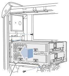
Reinstall the optical drive carrier in the computer. Make sure this guide engages the slot in the chassis. Push the carrier forward until it is firmly seated, and then tighten the two screws.
