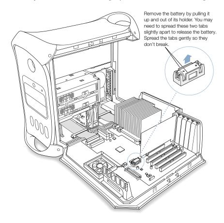
2 If necessary, carefully spread the tabs holding the battery so you can remove it.
