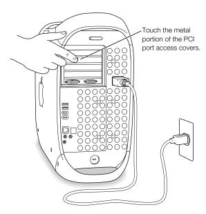
**Important** Always do this before you touch any parts, or install any components, inside the computer. To avoid generating static electricity, do not walk around the room until you have finished installing the expansion card, memory, or internal storage device and closed the computer.
