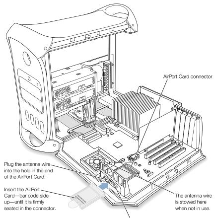
Tuck the clear plastic tab on the AirPort Card up into the slot in the card guide.
