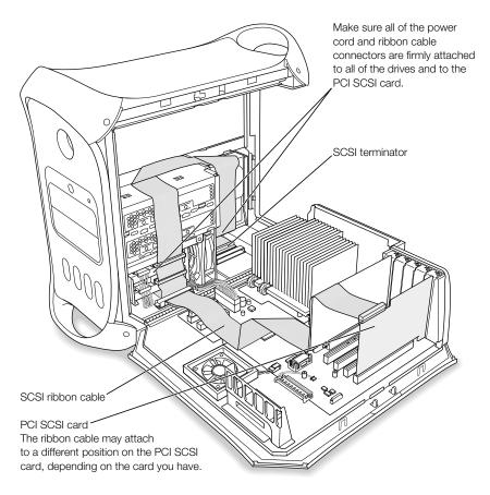
The procedures for disconnecting and connecting a SCSI hard disk drive and for removing and inserting drive carriers are nearly identical to those presented in the ATA drive installation instructions on page 74. Follow the ATA drive instructions when installing a SCSI drive.
