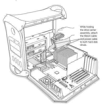
7 Replace the drive carrier on the chassis, pushing gently until it locks into position.
