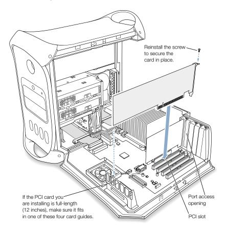
Press the card gently but firmly until the connector is fully inserted.
