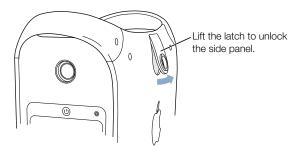
*Note:* If the latch won't lift, check that the security lock port and lockable cover latch in the back of the computer are not locked.
