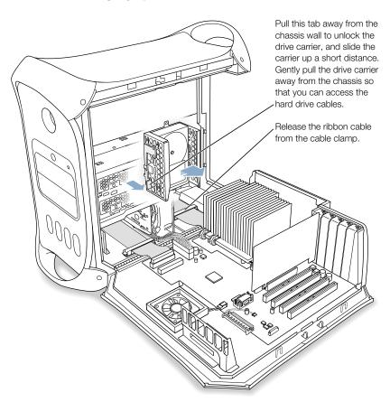
3 Release the cable from the clamp.
